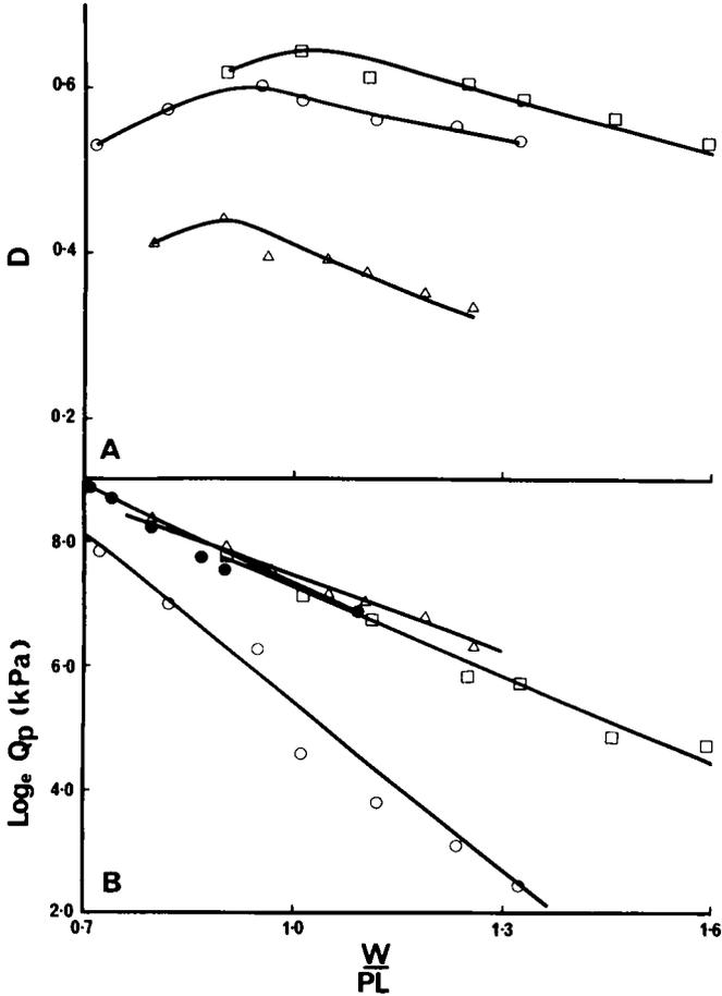
FIG. 1. Effect of water content at remoulding ( $W/PL$ ) on packing density,  $D$ , and penetration resistance,  $Q_p$ , of freshly-remoulded Urrbrae (○), Strathalbyn (□), and Waco soils (Δ), and penetration resistance of 'undisturbed' Urrbrae field clods (●). A. Packing density. B. Penetration resistance (the straight lines are fits of equation 3).
