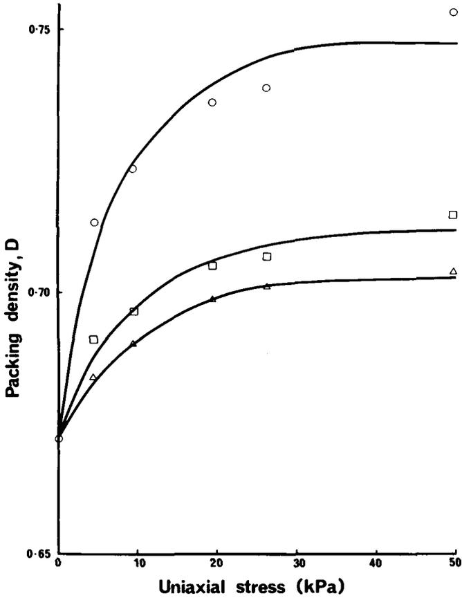
FIG. 5. Effect of ageing on the stress dependence of the compression resistance of Urrbrae loam. Measurements are given by: (O) non-aged; (□) 1 day; (△) 6 days, and the curves are fits of equation 5.
