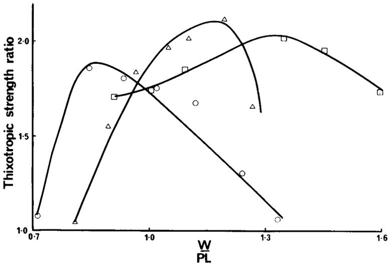
FIG. 4. Effect of water content at remoulding on thixotropic strength ratio of the Urrbrae (○); Strathalbyn (□), and Waco (△) soils after 12 days ageing.
