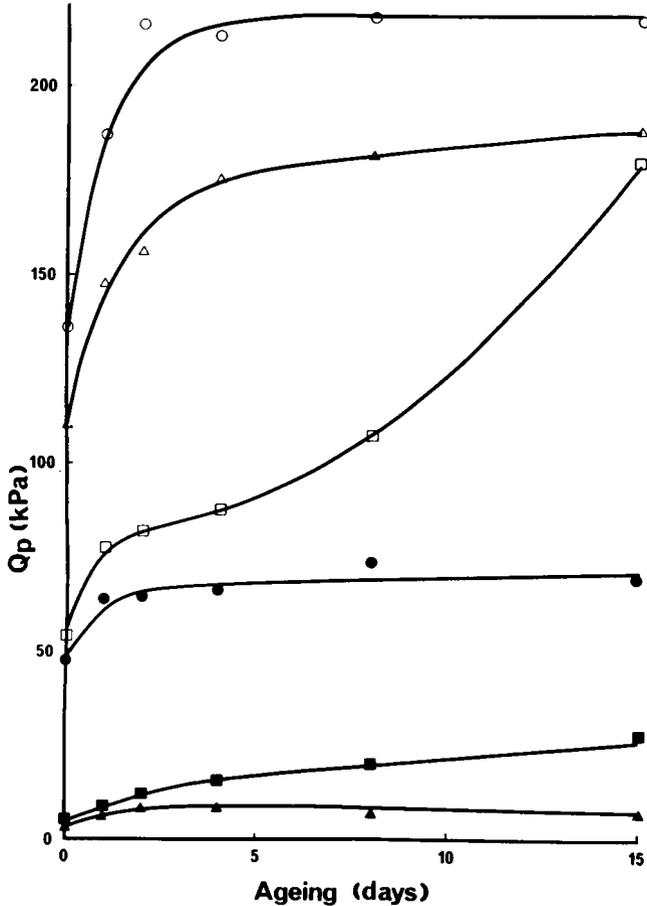
FIG. 2. Effect of ageing on the penetration resistance,  $Q_p$ , of the Urrbrae soil. (○) control 20 per cent water content; (●) control 22 per cent water content; (□) oxidized 20 per cent water content; (■) oxidized 22 per cent water content; (△) sterilized 20 per cent water content; (▲) sterilized 22 per cent water content.
