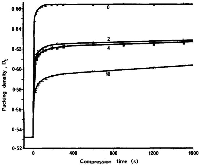
Fig. 3. Effect of ageing (0, 2, 4, 10 days) on the time dependence of the compressibility of beds of aggregates of Urrbrae loam when they are suddenly subjected to a uniaxial stress of  $S = 29.43$  kPa. Points are single measurements; the curves are from eq. (6).
