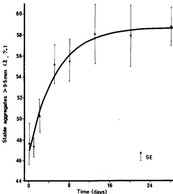
Fig. 1. Effect of ageing since disturbance on the water stability of aggregates of Urrbrae loam. Points are the means of three measurements; the curve is from eq. (4).
