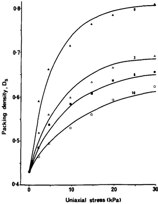
Fig. 2. Effect of ageing (0, 3, 6, 10 days) on the resistance to compression of beds of aggregates of Urrbrae loam. Points are single measurements; the curves are from eq. (5).
